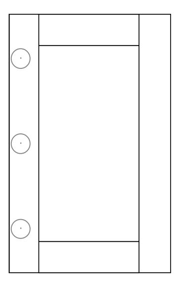
BORE PLACEMENT FOR DOORS 11" AND UNDER IS 2" FROM THE TOP AND BOTTOM OF THE DOOR TO THE CENTER OF THE 35MM BORE HOLE.
