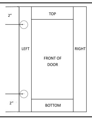
STANDARD BORE PLACEMENT IS 3 1/2" INCHES FROM THE TOP AND BOTTOM OF THE DOOR TO THE CENTER OF THE 35MM BORE HOLE.
